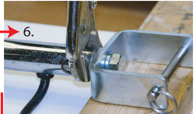
Crimp tube very hard with a wise grip to prevent the saddle moving
