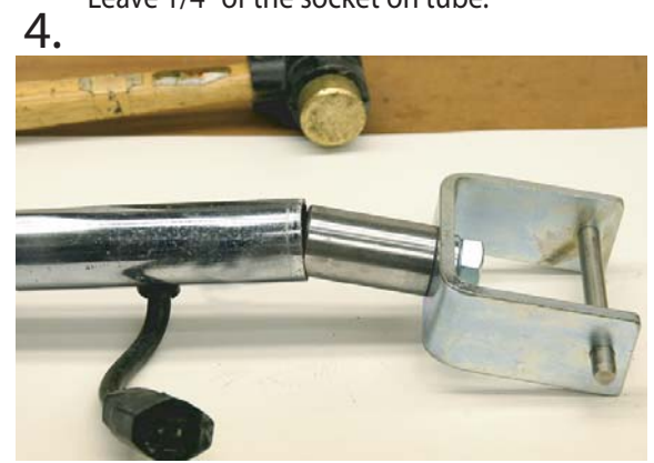
Insert Saddle assembly to tube opening.
