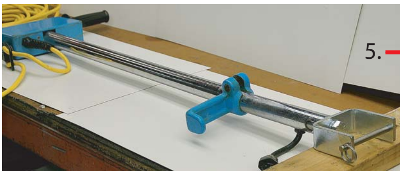
Lay it flat on a bench & let it rest on a 2x4 wood. The wood will give clearance to the protruding cable.
