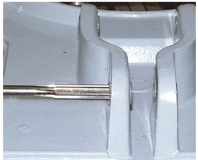
6. Ream it with 3/8" reamer either by hand or with drill at slow speed.
