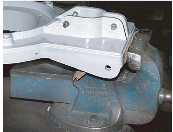
2. Put base in a vise and drive out old bushings with a 12mm or 3/8" punch. (Warning. The hole size in casting is 29/64" Your 1/2" punch may get stuck in it)
