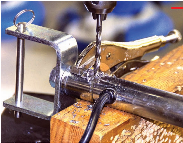
Drill hole with a size "D" drill bit (incl. in the kit)
