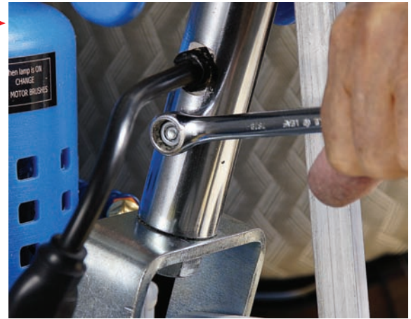
Place 1/4" bolt in hole, add flat washer and let the LONG side hang down then tighten the nut.
